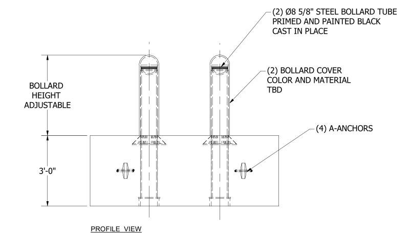
PART INFORMATION DESCRIPTION QTY APPROX. WEIGHT IN LBS 8,700 BP-2-3ft SPACING BASE 9,800 BP-2-4ft SPACING BASE BP-2-5ft SPACING BASE 10,900 8 5/8 OD STEEL BOLLARD TUBE N/A AND COVER
