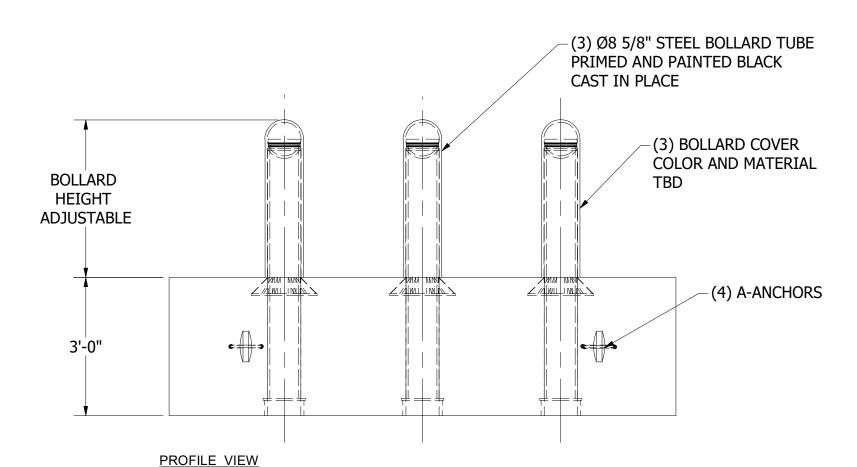
PART INFORMATION DESCRIPTION APPROX. WEIGHT IN LBS 11,900 BP-3-3ft SPACING BASE 14,100 BP-3-4ft SPACING BASE BP-3-5ft SPACING BASE 16,400 8 5/8 OD STEEL BOLLARD TUBE N/A AND COVER
